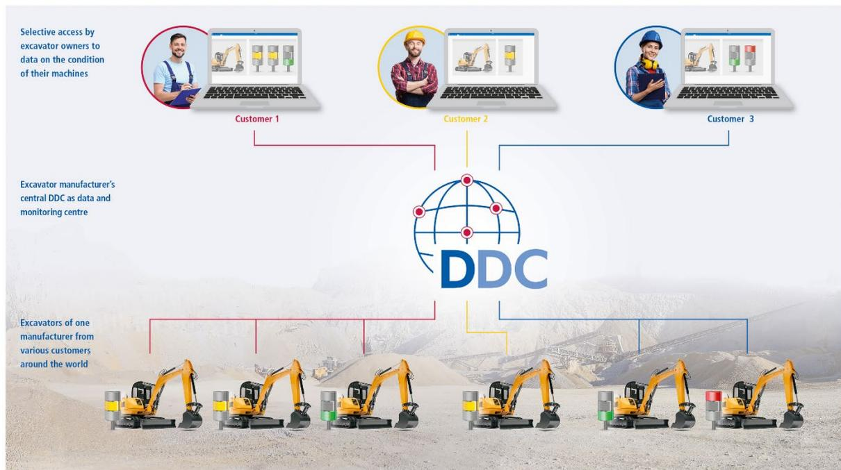
“Condition Monitoring as a Service”. A construction machinery manufacturer is providing condition monitoring as an additional service, thus creating significant added value for its customers. The solution has been implemented with intelligent ICA systems from Delphin for data acquisition, central measurement data management using the Delphin Data Center, and ProfiSignal 20 for location- and platform-independent visualisation.
